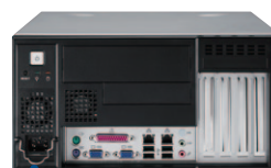
Plug ring-lock securely fastens the power cord
